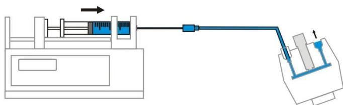
7. Subsequently connect a red-striped PEEK (127  $\mu\text{m}$  ID, 1/16" OD, typically 1 meter in length) outlet tubing to the outlet port of the cell using a 10-32 fingertight fitting. Fill the outlet tubing with sample solution.
