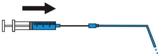
4. Connect the outlet of the tubing to the inlet of the  $\mu$ -PrepCell using a 10-24 fingertight fitting. Make sure that the outlet tubing and REF electrode are removed from the cell.
