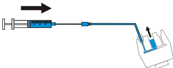
5. Check visually if there are no air bubbles present in the sample solution in the REF chamber. If any air bubbles are present try to remove them. Mount the REF electrode and make sure not to introduce any air bubble during the mounting process. Subsequently, continue filling the cell until the solution is siphoning (air bubble free) from the outlet port.
