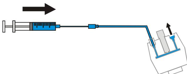
6. Place the syringe in the infusion pump and start the infusion pump to dispense at the designated flow rate.
