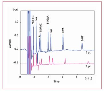
Figure 7: Effect of injection volume on chromatograms of 10 nmol/L standards in Ringers solution with 10 mmol/L acetic acid. Conditions as in Table 1, but with  $\mu$ VT-03 flow cell and ISAAC ref. electrode vs 8 mmol/L KCl (640 mV).
