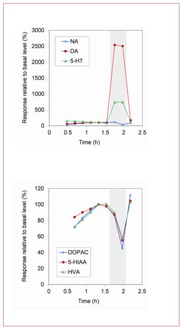
**Figure 12:** Response plots as obtained from an on-line coupled in-vivo brain microdialysis experiment. A sample split set-up was applied for parallel analyses with the ALEXYS Analyzer for OMD (applications for monoamines and acidic metabolites). The grey area in the graph indicates the time span when the perfusion fluid contained a high potassium concentration to induce a response.
