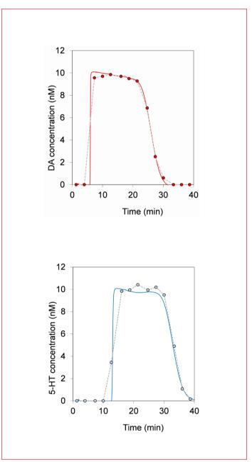
**Figure 11:** Fast changes in DA and 5-HT levels (red and blue colored profiles) are accurately measured with the ALEXYS Analyzer for OMD with High Time resolution option (dots and dashes).
