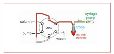
$\textbf{Figure 9:} \ Schematic \ representation \ of the \ 'probing' \ method \ in \ an \ on-line \ microdialysis \ set-up$
