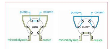
**Figure 4:** Connections at 2-positions 6-port valve for on-line microdialysis sampling.
