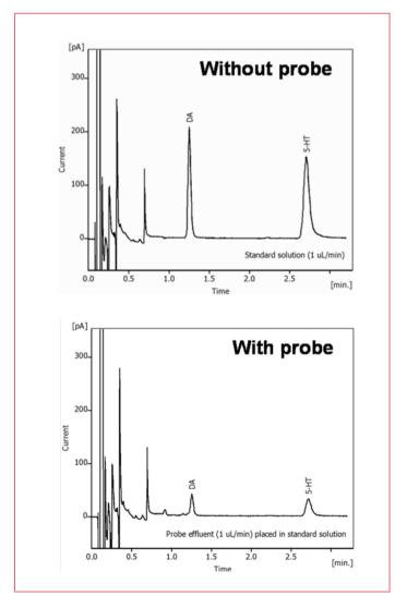
**Figure 10:** Two example chromatograms used for calculation of probe efficiency. A standard is directly analyzed or sampled through a probe in an online microdialysis coupled ALEXYS system. Probe efficiency was calculated to be 15-20% in this case.
