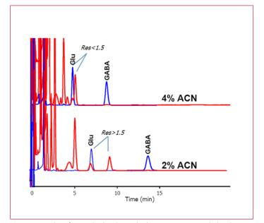
**Figure 5:** Overlay of a standard and sample chromatogram recorded with 2% or 4% acetonitrile in the mobile phase. Red trace: pooled rat dialysate from the Hippocampus. Blue trace: 5  $\mu$ mol/L GABA and Glu standard mixture in Ringer solution (separation and detection at 35 °C). With courtesy to Niels Leguit, Abbot Healthcare Products B.V., Weesp, the Netherlands for providing the samples.
