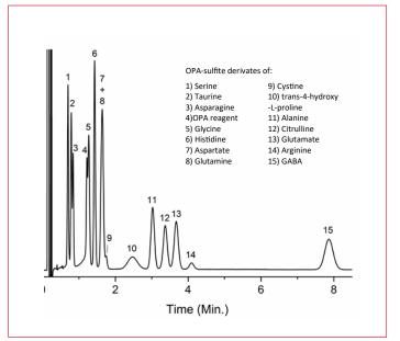
**Figure 4:** Chromatographic profile of OPA-sulfite derivatized standards mix of amino acids and related substances in water. Chromatographic conditions according to Table 1 (but with a mobile phase with pH set to 3.28 and 1% acetonitrile and 2 % methanol). With courtesy to Mrs. Gerdien Korte-Bouws, Department of Pharmaceutical Sciences, division of Pharmacology, University of Utrecht, The Netherlands.
