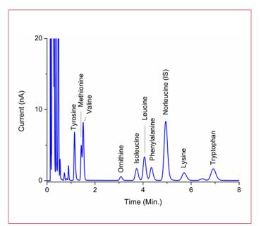
**Figure 16:** Analysis of extracted chicken plasma. Conditions according to Table 1, except the use of a flow cell with a 0.7 mm GC electrode and a mobile phase according to Table 5. Chromatogram courtesy of Mrs. Gerdien Korte-Bouws, Department of Pharmaceutical Sciences, division of Pharmacology, University of Utrecht, The Netherlands.
