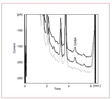
**Figure 12:** Analysis of a 2 nmol/L GABA standard prepared in Ringer solution (duplicate) in overlay with a blank (grey trace). Conditions according to Table 3. Chromatogram courtesy of Mrs. Lucy Pinder, RenaSci, Nottingham, UK.
