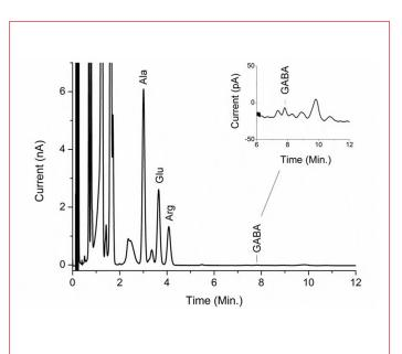
**Figure 13:** Chromatogram of microdialysate sample from a rat prefrontal cortex. The insert in the top-right corner is a zoom in on the GABA peak. Conditions according to Table 1, except the use of a flow cell with a 0.7 mm GC electrode and mobile phase with pH set to 3.28 and 1% acetonitrile and 2% methanol. With courtesy to Mrs. Gerdien Korte-Bouws, Department of Pharmaceutical Sciences, division of Pharmacology, University of Utrecht, The Netherlands.
