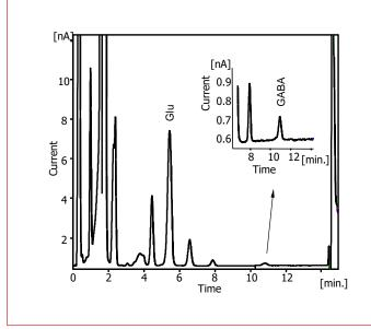
**Figure 14:** Chromatogram of microdialysate sample from a rat nucleus accumbens. The insert in the top-right corner is a zoom in on the GABA peak. Conditions according to Table 1, except the use of a flow cell with a 0.7 mm GC electrode. With courtesy to Niels Leguit, Abbot Healthcare Products B.V., Weesp, the Netherlands for providing the samples.
