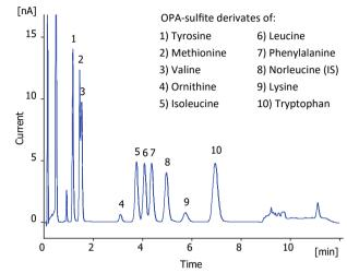
*Fig. 2.* Analysis of a 10 μM standard mix of 10 LNAAs and related compounds. Conditions according to Table 1. Chromatogram courtesy of Mrs. Gerdien Korte-Bouws, Department of Pharmaceutical Sciences, division of Pharmacology, University of Utrecht, The Netherlands.
