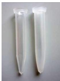
**NOTE:** There are subtly different shapes of fraction collector vials on the market. The types that fit best are the ones from Microbiotech, depicted on the left side in Fig. 1. The types depicted on the right are slightly too wide to fit in the 96-position tray; such vials can be sampled by placing them in adaptors that fit in the 48 positions tray. Reusable adaptors can be purchased at Antec Scientific (pn. 181.0726; Microdialysis coll. vial adaptors, 100pcs)
