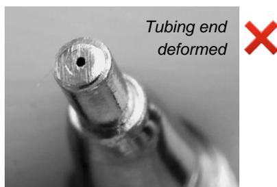
Fig. 1. Sleeved SS tubing leaks and shows deformation after tightening the nut with the tubing end bottomed into the receiving port.
