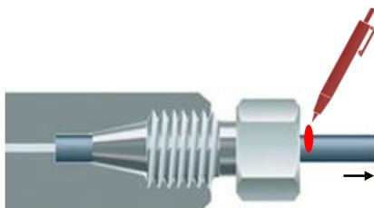
3. With a marker, draw a line at the point where the tubing goes into the nut.
