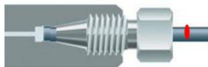
4. Retract the tubing **about 0.5 - 1 mm** and tighten the nut.
