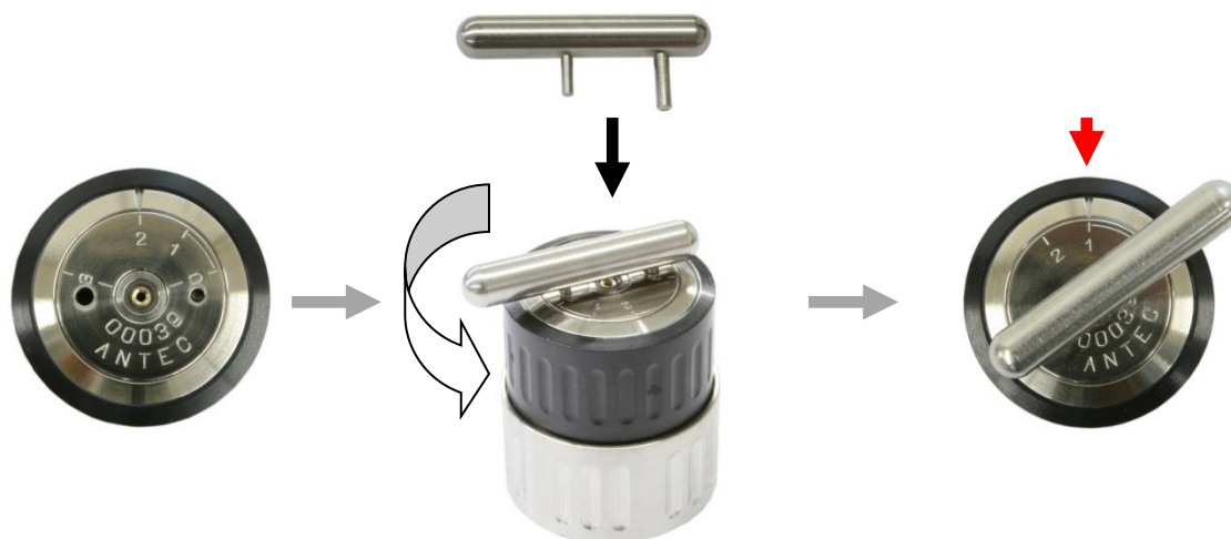
Fig. 10. Adjustment of the working volume from position 2 (left side) to 1 (right side).
