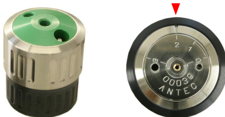
Fig. 9. Left side : photo of assembled SenCell inlet block (green) with In-Situ Ag/AgCl (ISAAC) reference electrode (REF). Right side : bottom side of the SenCell with the Cell working volume adjustment system, Auxiliary (AUX) electrode contact (opening on left side next to inscription '3') and Working electrode (WE) contact (opening in the center). The cell working volume is preset on position 2.
