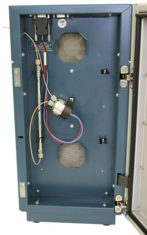
Fig. 11. Left : SenCell with ISAAC reference mounted under an angle of approximately 45 °C in the DECADE II detector. [1] Cell clamp, [2] Cell Inlet (tubing connection from column-to-cell), [3] Cell outlet (tubing connection from cell-to-waste) make sure that the outlet is positioned on the top side to prevent entrapped air bubbles, [4] WE contact (red), [5] AUX contact (blue), [6] REF contact (black). Top-right : electrical connections of WE (red connector) and AUX electrode (blue connector). Bottom-right : SenCell with Saltbridge reference electrode.
