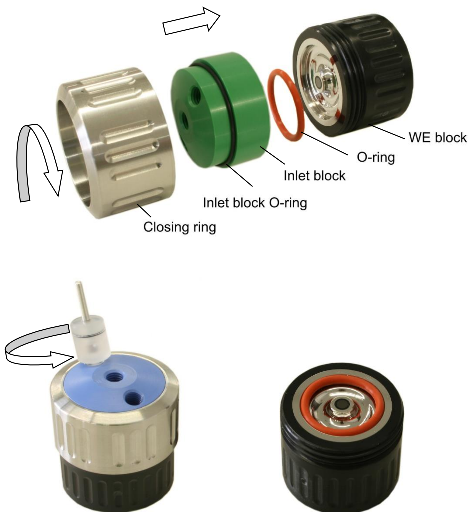
Fig. 14. Top: Exploded view of SenCell. The arrows indicate how to assemble the cell. Bottom left: unscrewing the Salt bridge electrode. Bottom right: WE block with O-ring placed in designated O-ring groove.
