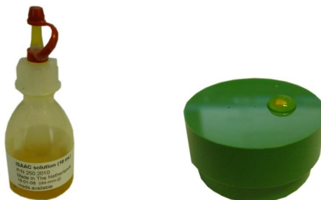
Fig. 16. Left : ISAAC solution. Right : ISAAC inlet block with a droplet of ISAAC solution applied on the freshly polished reference electrode.
