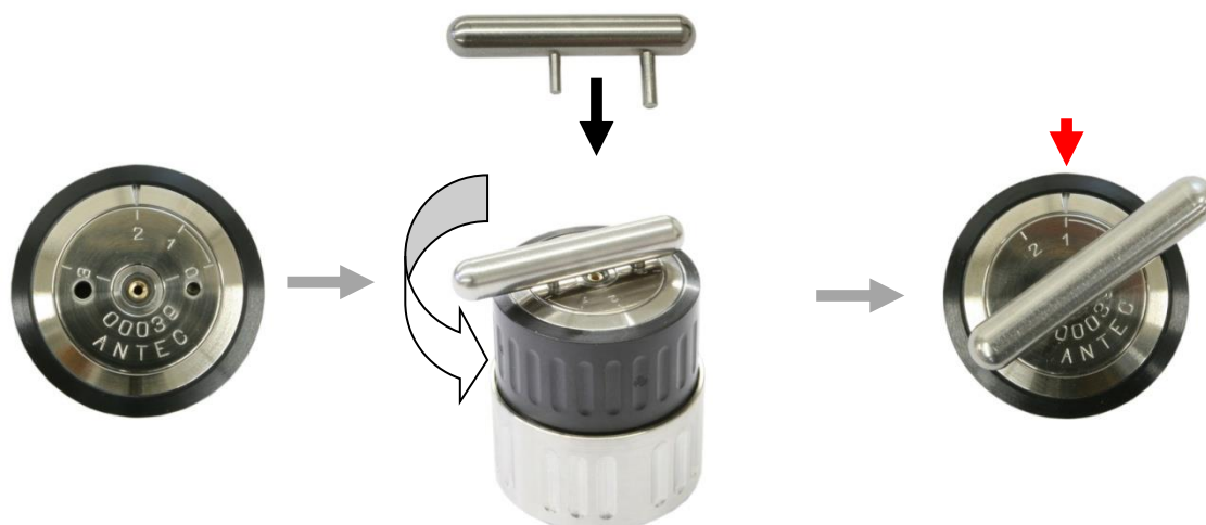
Fig 2. Adjustment of the working volume from position 2 (left side) to 1 (right side).
