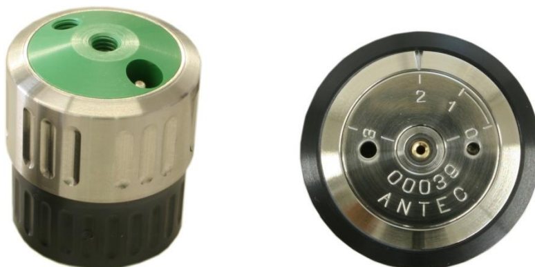
Fig 1. Left side: photo of assembled SenCell inlet block (green) with In-Situ Ag/AgCl (ISAAC) reference electrode (REF). Right side: bottom side of the SenCell with the Cell working volume adjustment system, Auxiliary(AUX) electrode contact (opening on left side next to inscription '3') and Working electrode (WE) contact (opening in the center).
