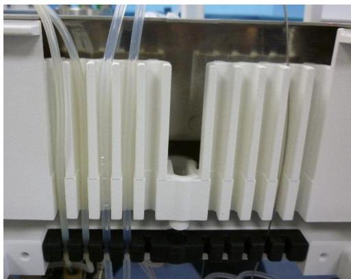
Figure 10. The tubing that is connected to the pump can be neatly organised behind the front panels of the pump and solvent tray.
