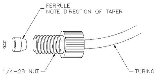
Figure 9. Assembly of 1/4-28 nut, ferrule and tubing for connection to degasser ports.
