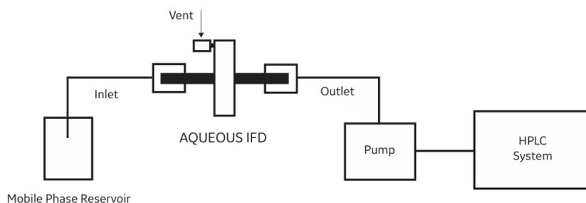
Figure 31. Schematic drawing of filter Installation in HPLC set-up. Do not insert the tubing too deep into the filter, as it could pierce through the membrane and damage the filter.
