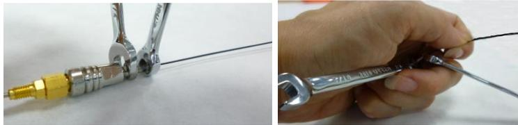
Figure 29. Internal 'through bore' reducer (1/32" to 1/16") being mounted on a pre-column filter. For clarity, the hands are not on the left photo, as the tubing needs to be held firmly bottomed into the port while tightening (the actual photo of how to hold everything is shown on the right – alternatively, do this with two persons or in a vice).
