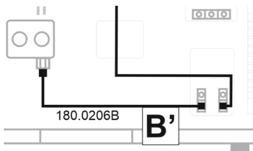
Figure 8. Connections at the degasser and pump inlet as pictured in the LC connections schematics. Note: on a P6.1L pump with integrated degasser, the assembly 180.0206B is already preinstalled.
