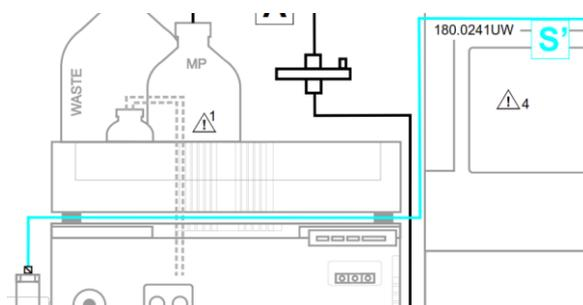
Figure 18. Connection at the pulse damper as pictured in the LC connections schematics for UHPLC systems.
