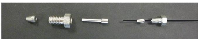
Figure 27. Exploded view of internal reducer (1/32" to 1/16") with the 1/16" nut and ferrule to the left, the 1/32" nut and ferrule mounted on the 1/32" OD PEEKSil tubing and the through-bore filler in the middle.
