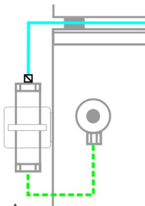
Figure 15. Connections between the pump purge valve and pulse damper as pictured in the LC connections schematics for UHPLC systems.
