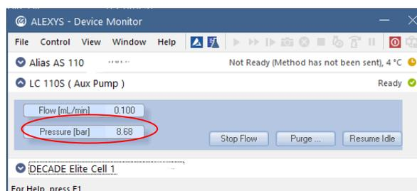
Figure 33. The Device Monitor window in Clarity software gives an accurate pressure reading.
