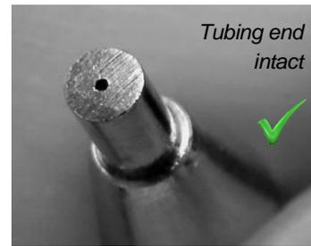
Figure 17. Sleeved SS tubing does not leak after installation with the described procedure.
