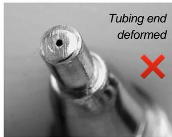
Figure 16. Sleeved SS tubing leaks and shows deformation after tightening the nut with the tubing end bottomed into the receiving port
