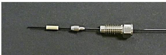
Figure 23. Assembly of PEEK sleeve, nut and ferrule onto 1/32" OD PEEKSil tubing for connection with a 1/16" receiving port.
