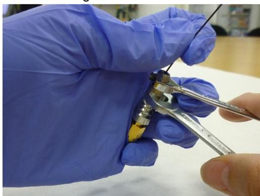
Figure 25. Connecting the 1/32" OD PEEKSil tubing to a prefilter with 1/16" receiving port requires holding the tubing into the bottom of the port while closing the nut with considerable force.
