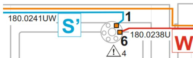
Figure 20. Connection at the injector valve as pictured in the LC connections schematics for UHPLC systems.
