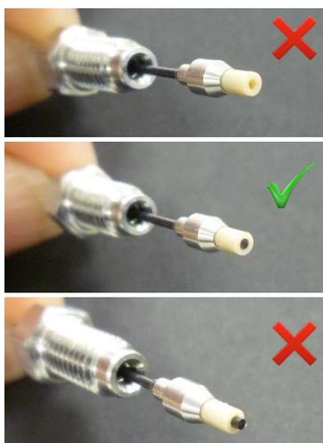
Figure 24. PEEK sleeve and PEEKSil tubing aligned correctly (middle), or incorrectly (top and bottom).
