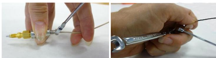
Figure 28. Filler, nut and ferrule being mounted on a pre-column filter while being held into place with a piece of 1/16" OD tubing. The second wrench to hold the pre-column filter in place is not shown on the left photo for clarity (the actual photo of how to hold everything is shown on the right – alternatively, do this with two person or in a vice).
