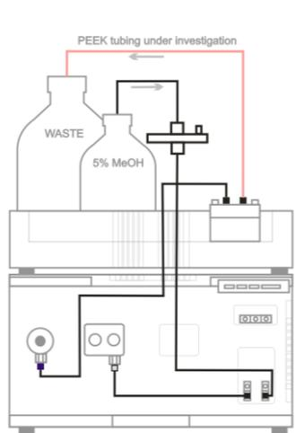
Figure 32. Configuration to determine the internal diameter of a piece of tubing by measuring the backpressure generated at a certain flow rate.
