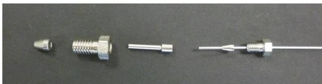
Figure 19. Exploded view of internal reducer (1/32" to 1/16") with the 1/32" nut and ferrule mounted on the 1/32" OD tubing
