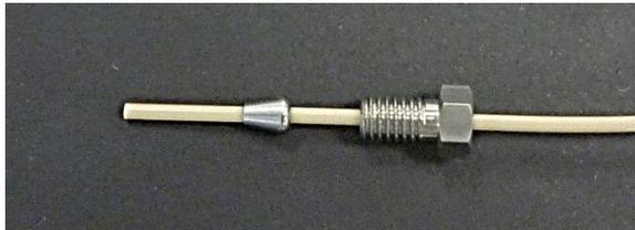
*Figure 11. Assembly of stainless-steel nut and ferrule onto 1/16" OD PEEK tubing.*
