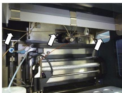
Figure 14. Picture of the autosampler with the waste tubing arranged through the valve compartment towards the waste bottle in the solvent tray.
