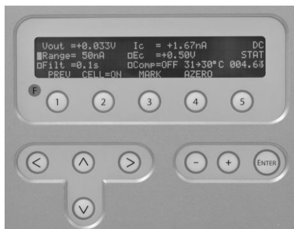
Fig. 3. ROXY Potentiostat keyboard. The cursor is on 'Range' which allows changes using the value buttons '+' and '-'. The 'Enter' button is only used to confirm changes in potential ( E_c ).
