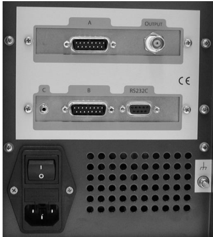
Fig. 26. ROXY Potentiostat rear panel.
