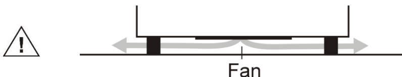
Fig. 2. Location of power supply fan DECADE II.
