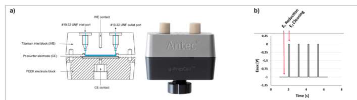
Figure 2: (a) Dual electrode \mu -PrepCell SS consisting of a Titanium inlet block and a Platinum counter electrode. (b) Applied pulse settings.
